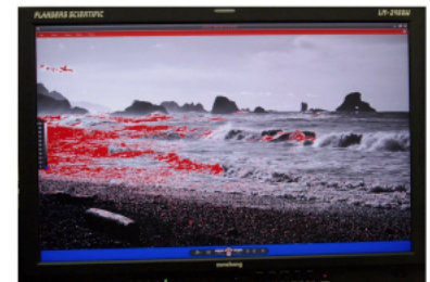
LUM Coloring with All Legal Levels Shown in Greyscale Underexposed Areas in Blue Overexposed Areas in Red
